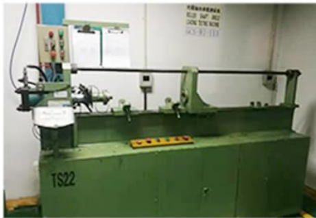
Axial bearing capacity testing bench
