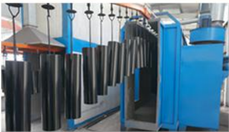
Roller automatic painting production line
