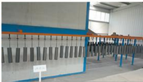
Roller automatic painting production line
